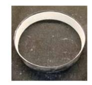
walls of the casting ring with 1/8" fiber strips. To avoid leakage and sticking, overlap the two cut ends of the strips and check to be sure fiber strips are sitting flat against kiln shelf.
