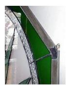
Joints are the best points to install the Handy Hanger. Using the edge of a half round bastard file, simply file a groove across the zinc. Insert the Handy Hanger tab into the groove up to the eye. Flux and solder.
