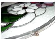
Using a generous amount of flux, flux notches and also the Hangers. Install Hangers and solder in place, being sure to solder closed any spaces.
