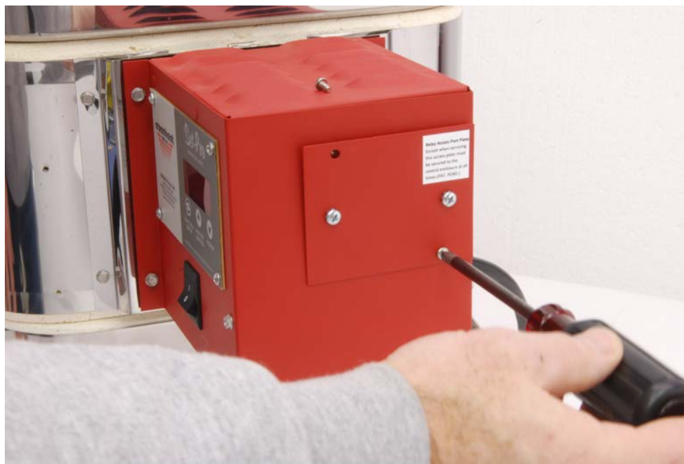
Remove the 2 screws that secure the relay access port to the control enclosure as shown.
