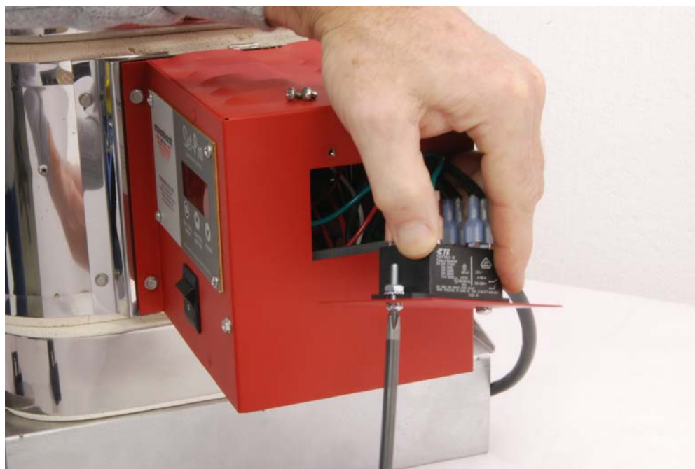
Attach the new relay to the relay access plate as shown.
