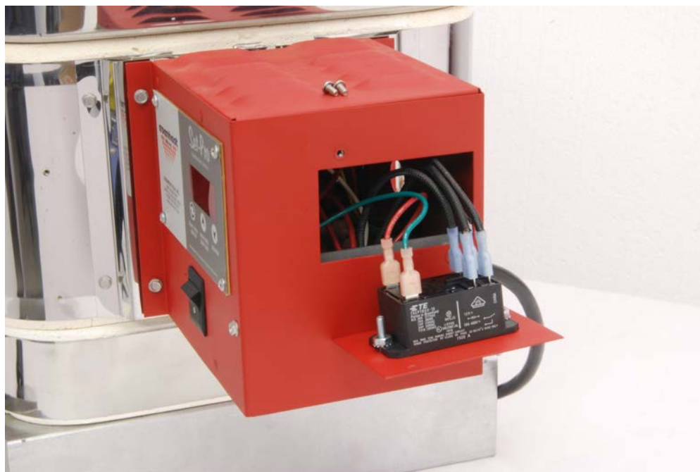
Pull the relay access plate away from the control panel to expose the relay as shown.
