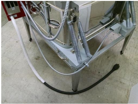
Route the conduit to back of stand as shown.
