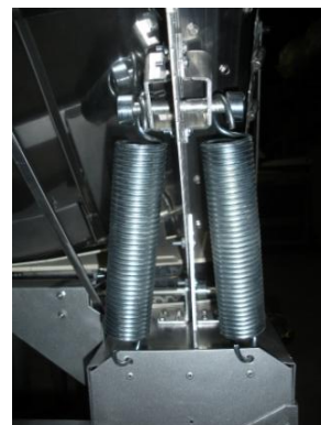
Properly placed lift assist springs, back left.
