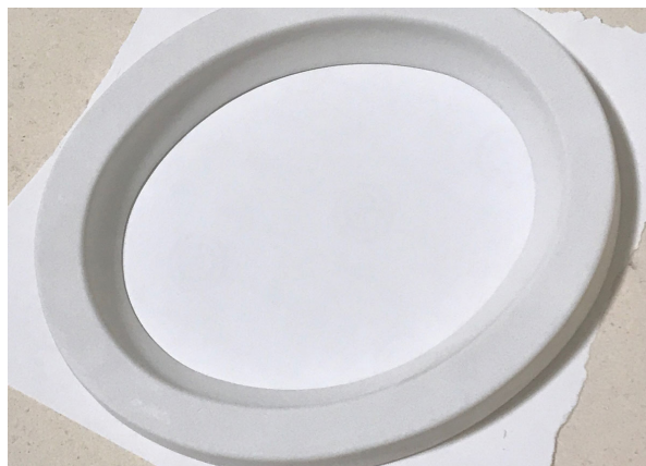
Place the Oval Shelf ring onto a piece of kiln shelf paper. Center the fused glass over the ring on the shelf and fire using the firing schedule found in Table 3*.
