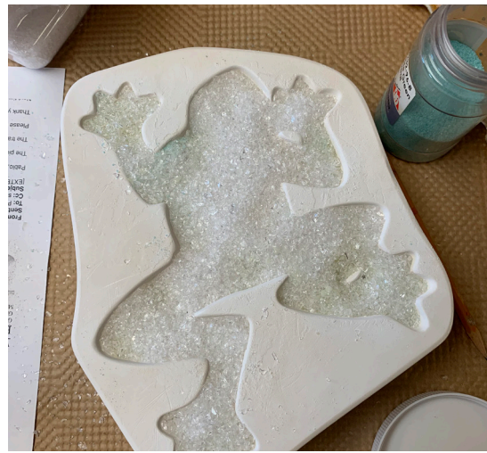
Place some F2 Clear into the body of the frog until the mold contains 326 grams of frit.
