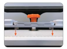
Turn off Grinder. Center THE SET horizontally across the Lift Grid, in-line with the grinding bit.
