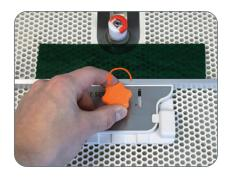
Tighten the Adjustment Knob by turning clockwise until it locks when the Adjustable Plate is in desired location. Remove glass piece.
