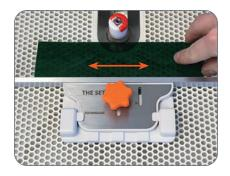
**6.** Place glass flush against aluminum bar and grind moving glass from **right** to **left**.
