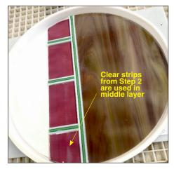
4. Prepare the mold by spraying with Boron Nitride and lining with a Papyros circle cut to fit. Place layers into mold as follows: color layer on the bottom (narrow window-border strips on-edge), then segmented clear layer in the middle with the clear intact circle as the cap. Full Fuse then slump, color-side up, into Colour de Verre 7-10" Bowl Slump Form. (Note that we opted to sandblast the surface of the bowl before slumping.)
